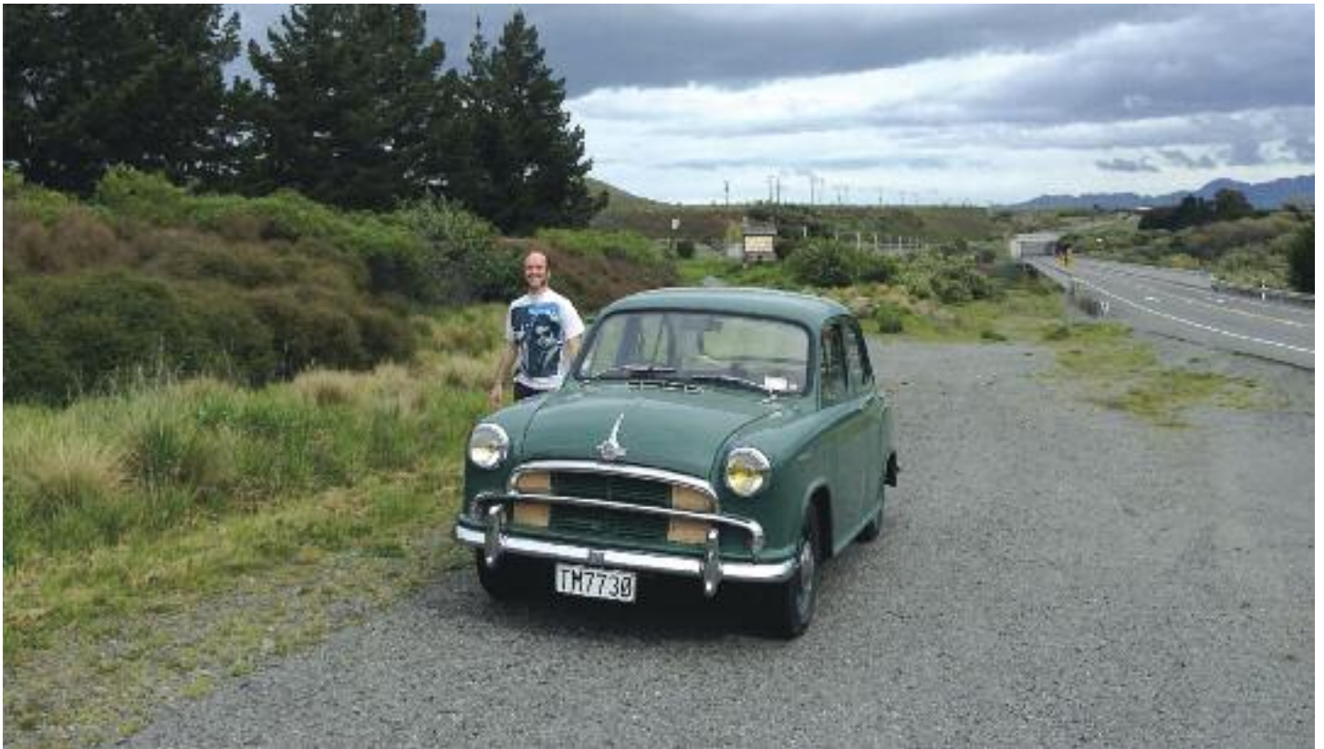
The Cowley and I beside the Awatere road/rail bridge, State Highway 1, close to Blenheim. These days road traffic has a separate two lane bridge; before this trains ran overhead and a single lane for all road traffic ran underneath. The cardboard muffs either side of the radiator are an attempt to force more air through the radiator because the temp gauge reads hot and there was pinking.
