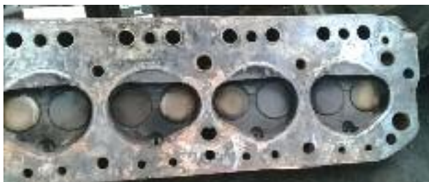
The original cylinder head with the Westlake Promontories completely ground away.
